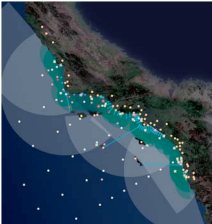
Fig.4. A large coastal ocean observatory consisting of short and long range CODARs and a diverse mix of buoys and short cabled observatories.
