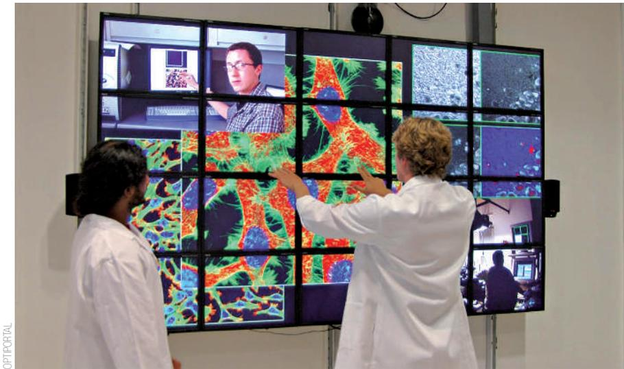
**Figure 1** An OptiPortal tiled display wall. Such lambda-connected displays enable researchers to view local high-resolution images at the same time as high-definition images from remote labs or computers in real time. Photo courtesy of David Lee, National Centre for Microscopy and Imaging Research (NCMIR) at UCSD.
